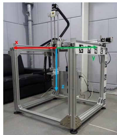
Fig. 1: Image of the robot with coordinate axes and mounted ArUco markers for precision measurement. The coordinate system utilized is a left-handed coordinate system.
