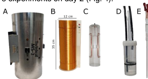
Fig. 2: Setup used for the experiment: (A) \mu -metal shield (Twinleaf MS-2), (B) In-house built B_0 -coil, (C) In-house built B_1 -coil, (D) water bath for temperature control, (E) high-pressure NMR-tube with capillaries for bubbling parahydrogen.
