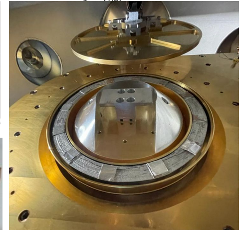
"floating coil" (sitting in cryostat, ready for cooling/quench tests)
